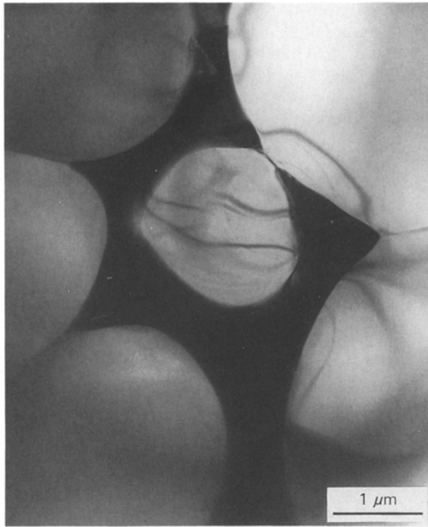
Figure 4 Bright-field TEM micrograph showing the morphology and location of the grain boundary phase from specimen LC sintered at 1810°C for 2 h.
